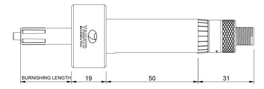
"Total length out of the chuck" is equal to ["burnishing length" + 19 mm]
